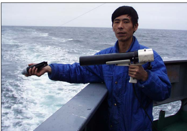
Expendable bathythermographs sample the structure of the upper layers of the ocean.
